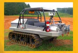
rubber track system that significantly reduces ground pressure, and can handle some of the most challenging terrains and swamps on the planet. Two hydraulically driven propellers at the rear of each Hydratrek ensure that deep water crossings will not slow down your operation.
